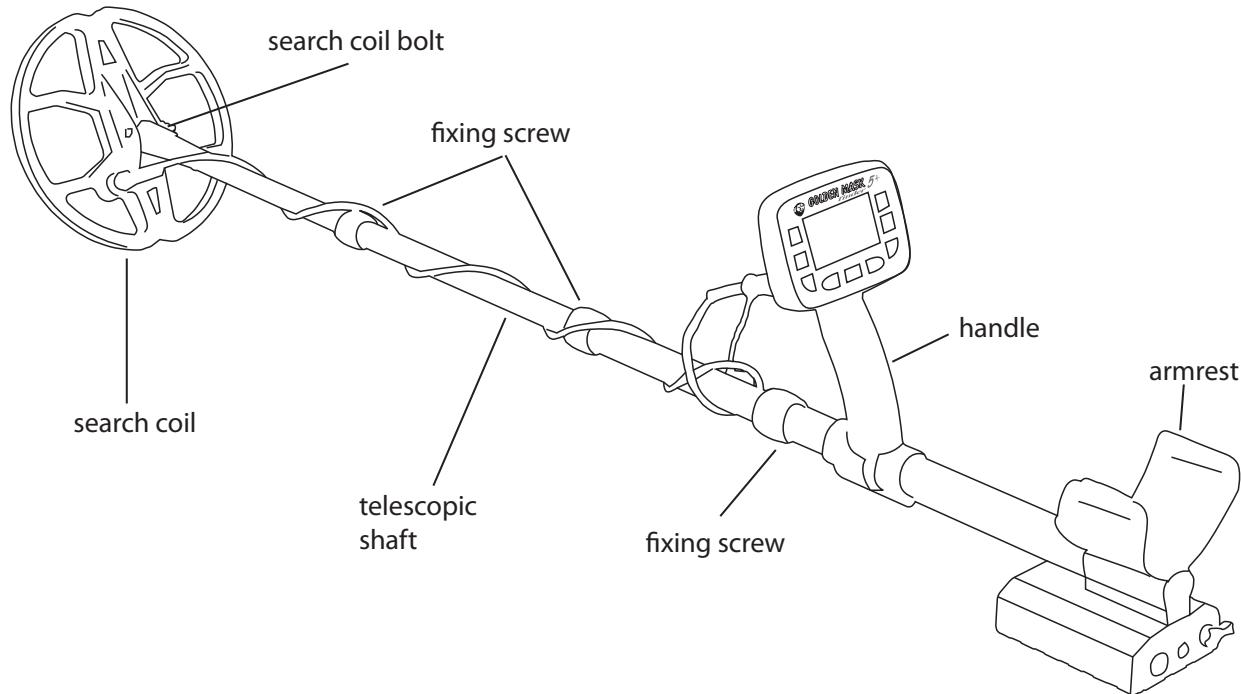
To extend the telescopic shaft, start from the first section (by the side of the coil). Turn the fixing screw counter-clockwise, pull the search coil gently to the full extent of the carbon pipe and then fix the section by gently turning the locking screw clockwise. Do the same with the second section. Check if the length is enough, if not, extend the third section to match the desired length.
